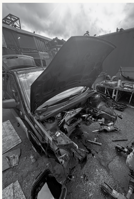
The prototype car's engine and fuel system were removed before any construction could begin. ©Pia Watson
