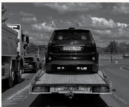
The cars are structurally designed to survive being transported with full water tanks. However, to avoid stress for the vehicle or drivers, they are moved with the minimum volume necessary to ensure that the filters remain submerged. ©David Cotterrell
