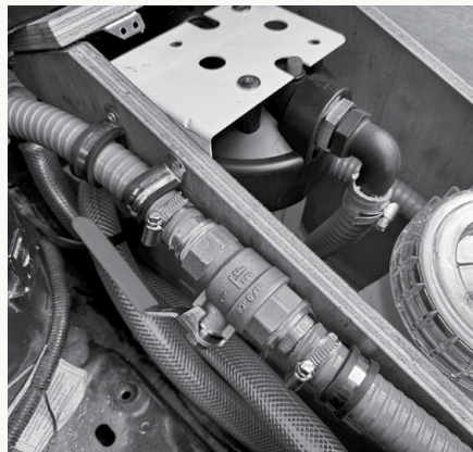
A weed-filter and canister filter process the water as it is drained from the cabin to the reservoir. The final-stage UV filter is hidden behind the grill of the engine bay. ©David Cotterrell
